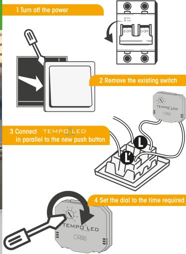
5 Mount the push button and TEMPOLED assembly into the installation box
